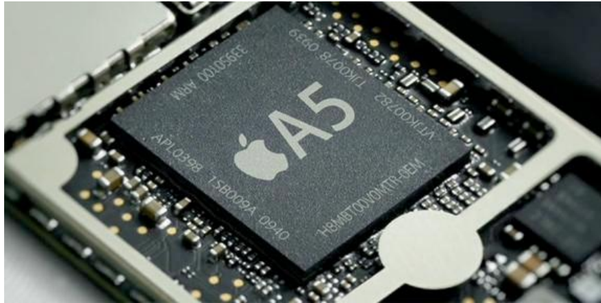
Apple A5: (in iPhone 4s and iPad 2) Dual Core CPU + GPU + image processor and more
